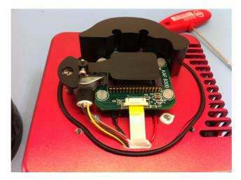
Carefully rotate the shutter to uncover the CCD
