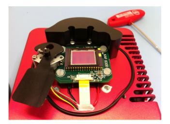
Dust can be removed from the sensor by blowing the surface gently with a camera lens "bulb" type cleaner but be careful not to introduce more dust from the surrounding area.
