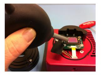
Thoroughly clean the CCD chamber to remove any material introduced and blow out the chamber using compressed air if possible.
